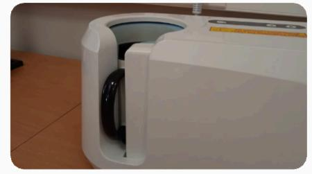
4. After transferring the ink, the material is cooled, causing the ink to condense back into a solid on the surface of the material. The print becomes permanent and resistant.
